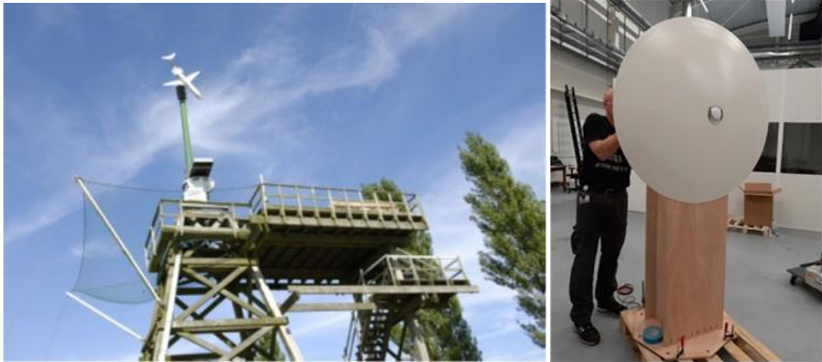
Figure 17: NLR's antenna test range (left), Ground plane and DPA on pedestal (right)
