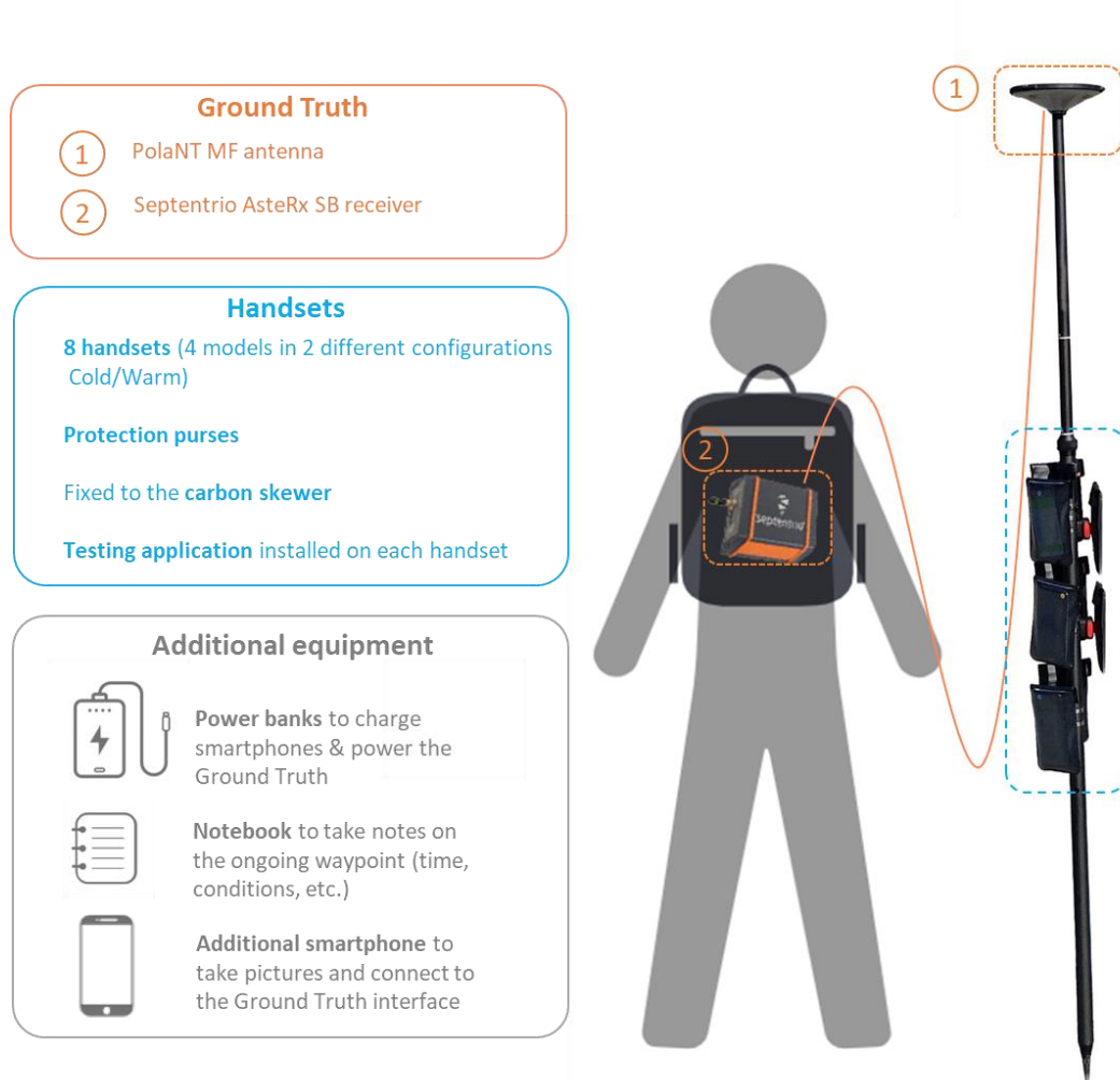
Figure 5-2 – Testing board for Help112 II project
