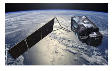
The satellite payload consists of three more instruments to enable the precise determination of the satellite orbit, namely a Global Navigation Satellite Systems (GNSS), a Doppler Orbit determination and Radio-positioning Integrated on Satellite (DORIS) assembly and a Laser Retro-Reflector (LRR). These instruments are all used to ensure the performance, accurate positioning and calibration of the SRAL products.
