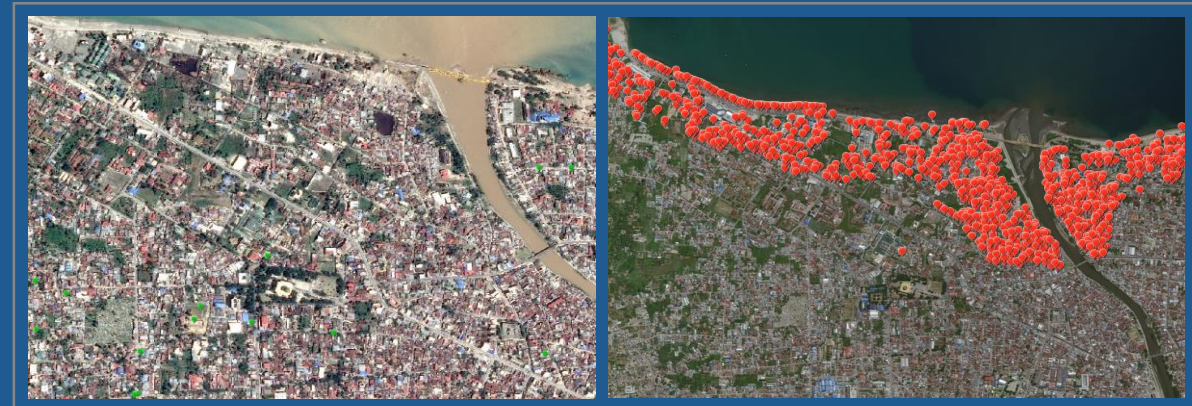
Optical view of the area affected by the tsunami (left) and analysis of building damages in the area affected by the earthquake and the tsunami (right) (Source: AIT)
