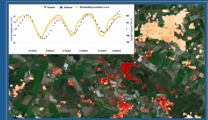
Correlation among gas injected volumes and measured deformation by the use InSAR analysis derived from Sentinel-1. Red points have higher correlation. Graph compares gas volume I/E with INSAR measures (Source: e-Geos)
