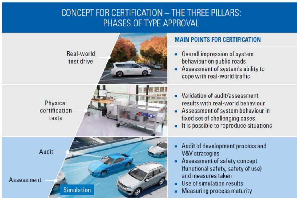
Figure 33 – Three pillars needed for ADAS type approval scheme according to TUV and dSPACE in order to cover requirements of UNECE R157 2 .
